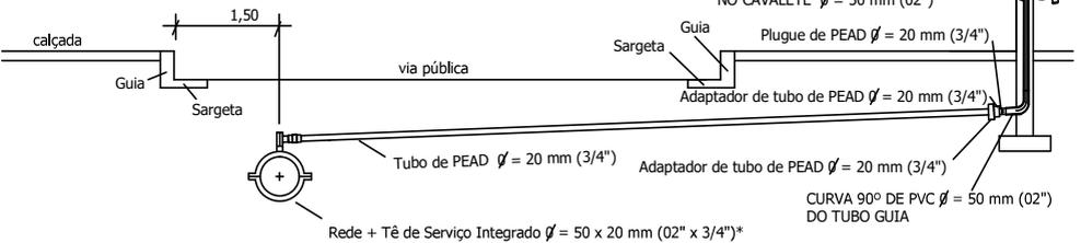
CURVA 90° DE PVC  $\phi = 50 \text{ mm (02")}$  DO TUBO GUIA
